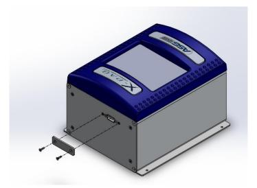
Align the 9-pin port of the ASG-NW2500 to the mating port on the top of the X-PAQ<sup>TM</sup> controller, connect, and tighten 4 screws.
